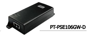
PT-PSE106GW-D is designed for indoor use. It works with input voltage of 32-72 Vdc. It has detection chip inside, which will detect and classify PD before powering it. It will not apply power until a standard-compliant PD is detected. The effective distance is 100 meters over Cat5e/Cat6 cables.
