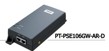
PT-PSE106GW-AR-D is designed for indoor use. It works with input voltage of 36-72Vdc. It has detection chip inside, which will detect and classify PD before powering it. It will not apply power until a standard-compliant PD is detected. The effective distance is 100 meters over Cat5e/Cat6 cables
