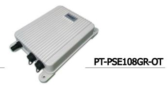
PT-PSE108GR-OT is designed for outdoor using, which works with 100-240Vac input and operates under -40°C to +65°C full loading. It has detection chip inside, which will detect and classify PD before powering it. It will not provide power until a standard-compliant PD is detected. The effective distance is 100 meters over Cat5e/Cat6 cables. It is specially suitable for working in complex power situations. It is easy to install with installation kit PT-POT-MBK, no need to open equipment.
