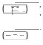
1.PoE Input Port2.Data Indicator3.Power Indicator4.USB-C Output Port
