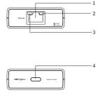
1.PoE Input Port2.Data Indicator3.Power Indicator4.USB-C Output Port
