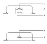
1.PoE Input Port2.Data Indicator3.Power Indicator4.USB-C Fixed holes5.USB-C Output Port
