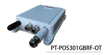
PT-POS301GBRF-OT is designed for outdoor using. It works with input voltage of 100-240Vac and operates under -40°C to +65°C. It has detection chip inside, which will detect and classify PD before powering it. It will not provide power until a standard-compliant PD is detected. The effective distance is 100 meters over Cat5e/Cat6 cables.
