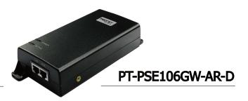
PT-PSE106GW-AR-D is designed for indoor use. It works with input voltage of 36-72Vdc. It has detection chip inside, which will detect and classify PD before powering it. It will not apply power until a standard-compliant PD is detected. The effective distance is 100 meters over Cat5e/Cat6 cables.
