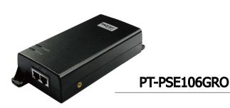
PT-PSE106GRO is designed for indoor use but can work outdoor by covered with waterproof case. It works with input voltage of 100-240Vac and operates under -40  $\degree$  to 65  $\degree$ . It has detection chip inside, which will detect and classify PD before powering it. It will not apply power until a standard-compliant PD is detected. The effective distance is 100 meters over Cat5e/Cat6 cables.
