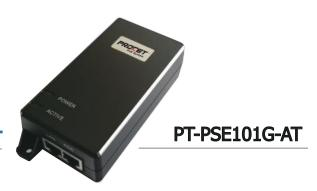
PT-PSE101G-AT is designed for indoor use. It works with input voltage of 100-240Vac. It will directly power PDs without detection. The effective distance is 100 meters over Cat5e/Cat6 cables.
