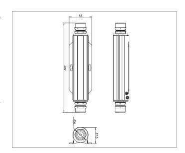
Order Info. PT-PEX-01G-OT 44-57Vdc(Max 60Vdc)/60W/1000Mbps/6KV Surge Protection/IP67/Outdoor use
