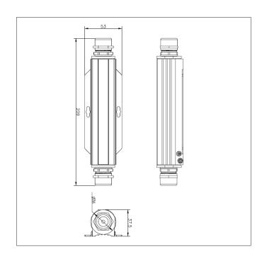
Order Info. PT-PR01G-OT 44-57Vdc(Max 60Vdc)/100W/1000Mbps/10KV Surge Protection/IP67/outdoor use
